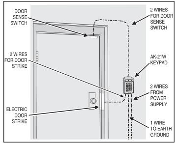
Figure 7. Basic Door Installation
